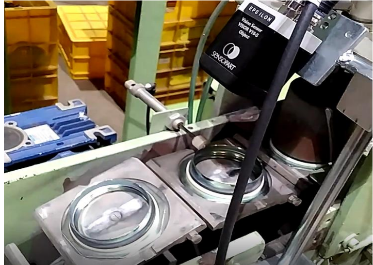
VISOR V10-S is deployed 110 mm from its target for detection of missing black or white/ twist/ flanges without gasket
